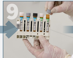
9 Take processed QC rack from unload tray and replace caps.
